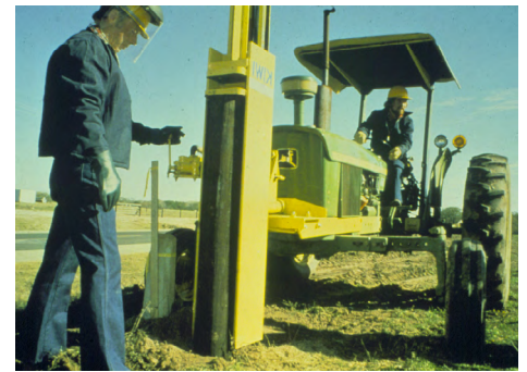
Figure 11. A tractor-mounted post driver.
